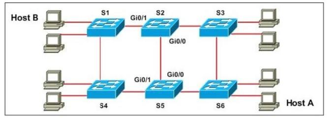
A. Yes. Traffic can pass either from switch S6 to S3 to S2 to S1, or, from switch S6 to S5 to S2 to S1.
